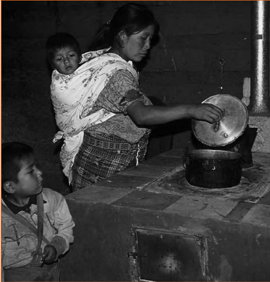
Figure 4.2 The 'plancha' wood stove. The combustion chamber is enclosed, and the cooking surface is made of steel with three pot holes at waist height. Although the hot surface and pots are out of reach of young, walking children, babies (carried on the mother's back while cooking) sometimes reach out and touch hot metal surface. Source: Nigel Bruce
