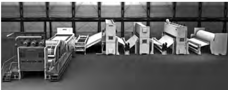
F4. Main equipments of AAT needle punching line
