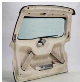
The 3D-Lighttrans tailgate created for the Fiat 500L (front).
