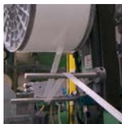
Sample: Selvage thread let-off SULEX guarantees a constant warp tension.
