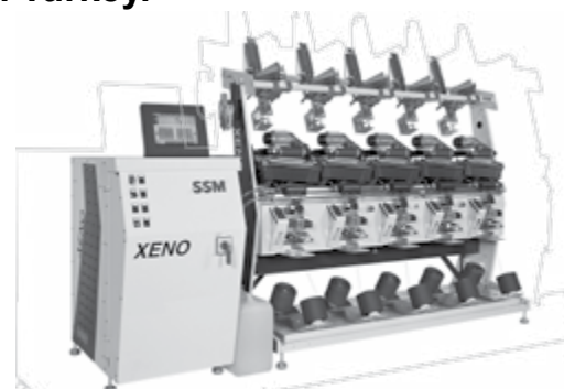
SSM XENO-YW precision package winder with DIGICONE® 2
