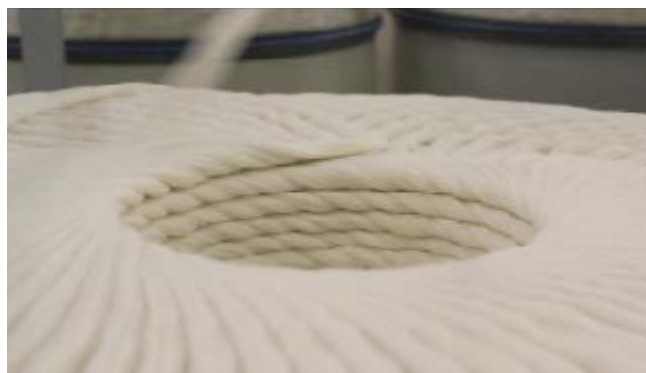
Figure 8: Picture of C701 card sliver
