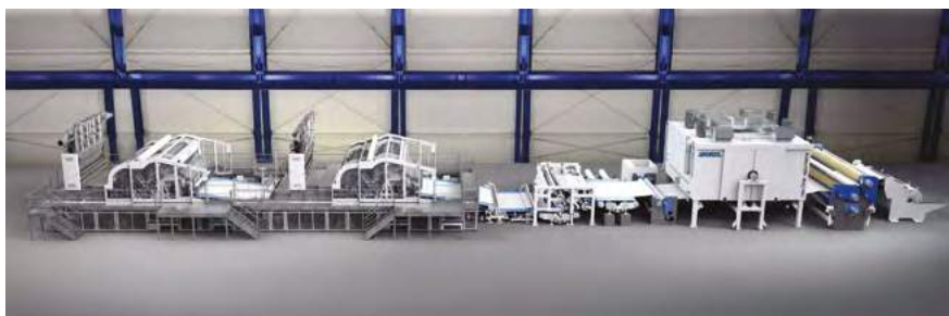
Fig 6 – ANDRITZ neXline Spunlace eXcelle Designed for the Production of Light Weight Spunlace Fabrics at Very High Speed
